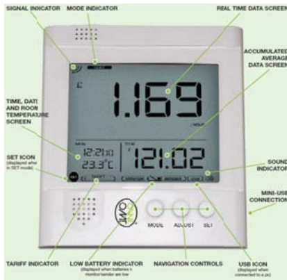
Figure 0-58: OWL metering receiver and Figure 0-59: OWL metering system: All-in-One: Metering and radio transmitter
