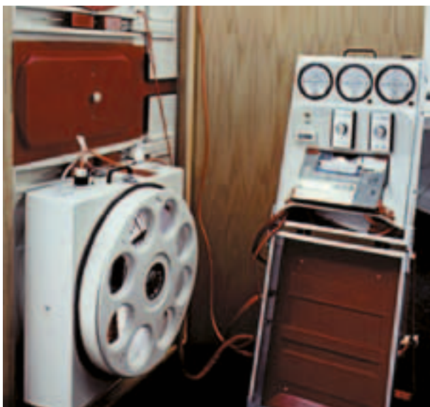
Blower door device to check the building's airtightness.
