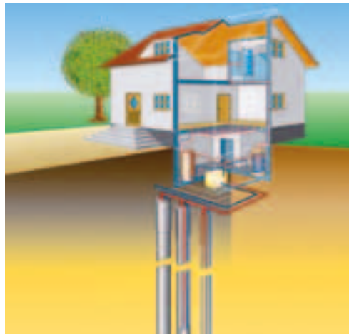
Heating system using a heat pump and geothermal probe to make use of ambient heat
